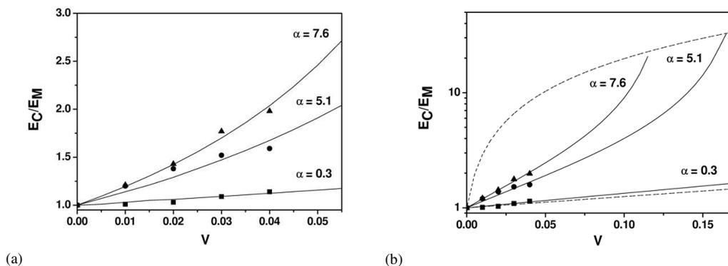
Fig. 3. Relative elastic modulus of LLDPE silica micro- and nanocomposites as a function of the filler volume content. (■) LLDPE-Glass-x, (●) LLDPE-A200-x, (▲) LLDPE-A380-x. (a) Fitting of experimental data according to the proposed model (continuous line, Eqs. 3-5); (b) comparison with the upper and lower limits according to Eqs. 1, 2 (dashed line).
