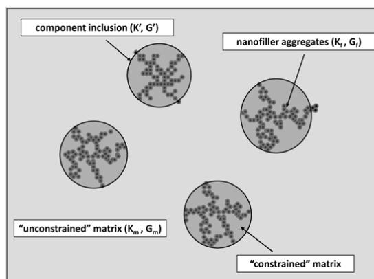
Fig. 1. Schematic representation of the structure of a particulate composite with primary particle aggregation.
