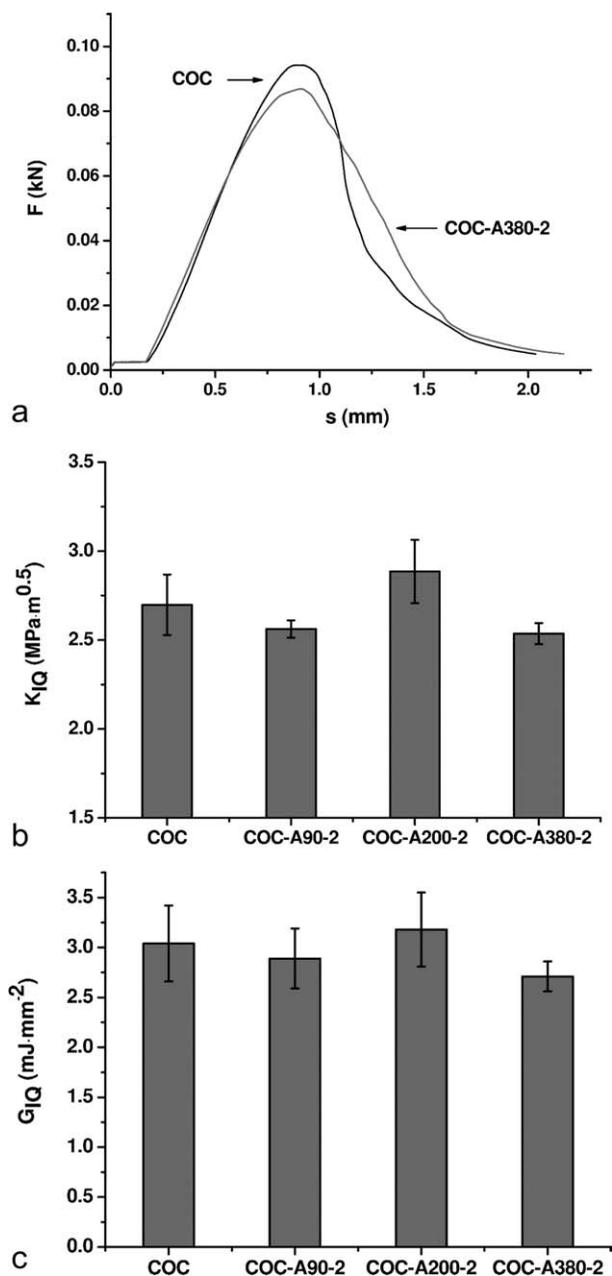
**Figure 8** Flexural tests of the single-edge notched samples for the determination of the fracture toughness of the COC and related nanocomposites ( $v = 10$  mm/min): (a) representative force–displacement curves, (b) apparent values of  $K_{IQ}$ , and (c) apparent values of  $G_{IQ}$ . “F” is the force and “s” is the deflection of the samples registered during the flexural tests.
