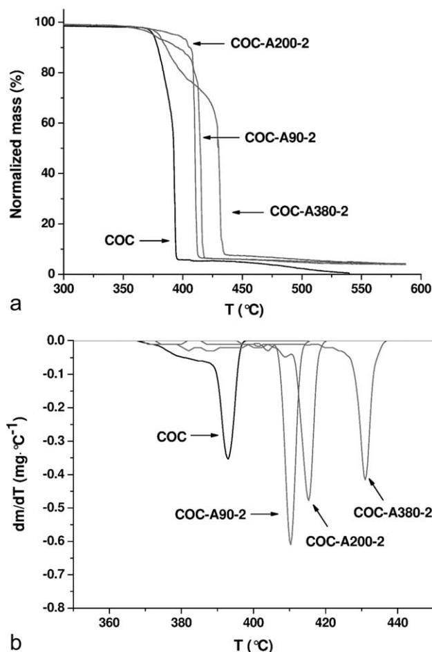
**Figure 4** TGA tests on the neat COC and related nanocomposites in oxygen atmosphere: (a) thermogravimetric curves and (b) derivative of the mass loss as a function of the temperature. “m” is the remaining mass during the TGA test.
