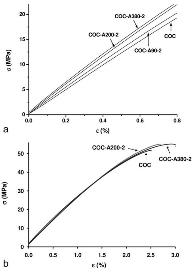
**Figure 6** Representative stress–strain curves of the neat COC and related nanocomposites in quasi-static tensile tests ( $v$ , crosshead speed = 1 mm/min): (a) evaluation of  $E$  and (b) evaluation of the tensile properties at break.
