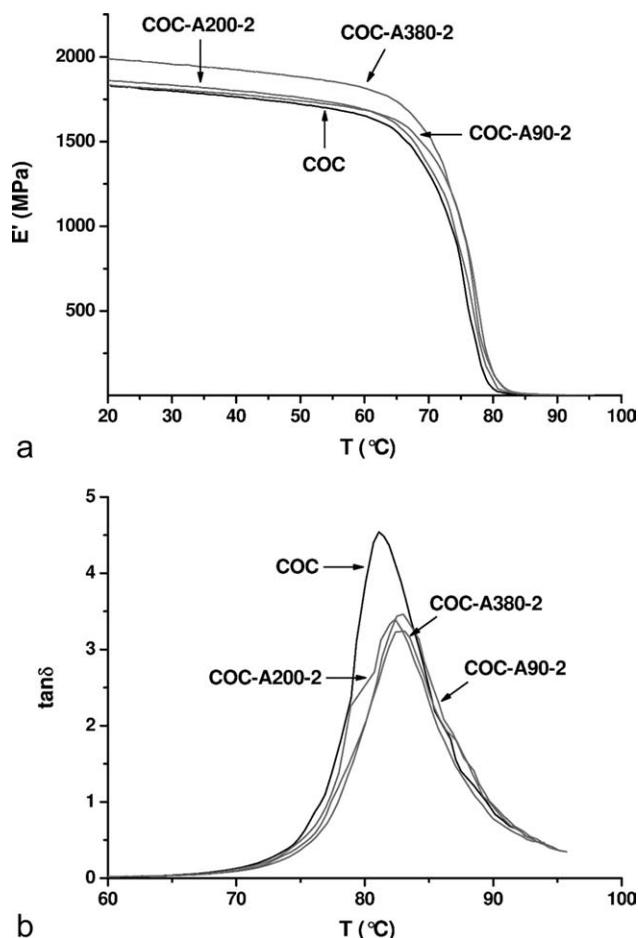
Figure 5 DMTA tests of the neat COC and related nanocomposites (frequency = 1 Hz): (a)  $E'$  and (b)  $\tan \delta$ .
