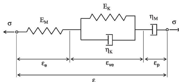
**Figure 2** Schematic representation of the Burgers model.  $\sigma$  = applied creep stress;  $\varepsilon_e$  = elastic component of the creep strain;  $\varepsilon_{ve}$  = viscoelastic component of the creep strain;  $\varepsilon_p$  = plastic component of the creep strain;  $\varepsilon$  = creep strain.
