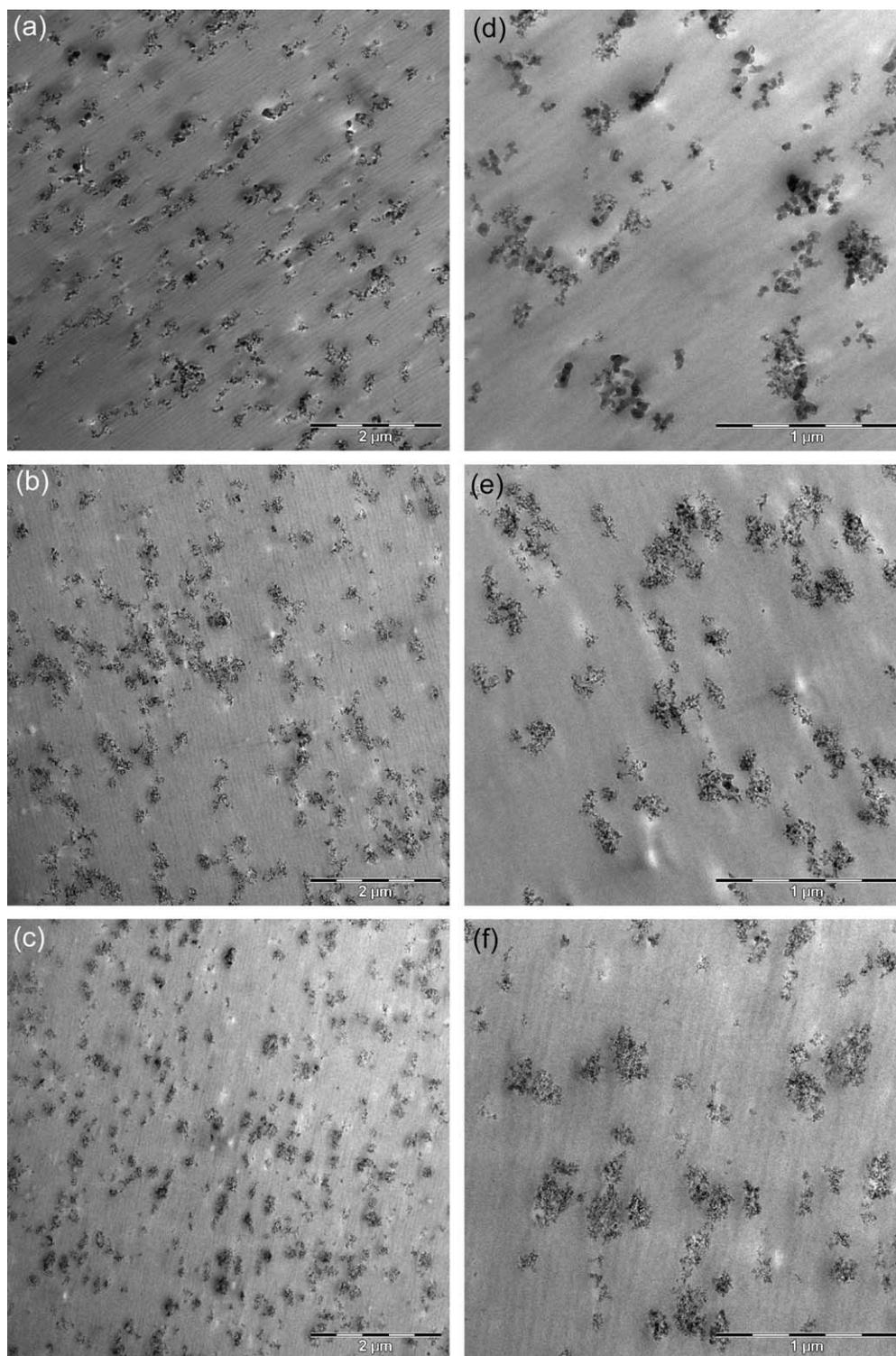
**Figure 3** TEM images of the COC/fumed silica nanocomposites at different magnifications: (a–d) COC–A90-2, (b–e) COC–A200-2, and (c–f) COC–A380-2.
