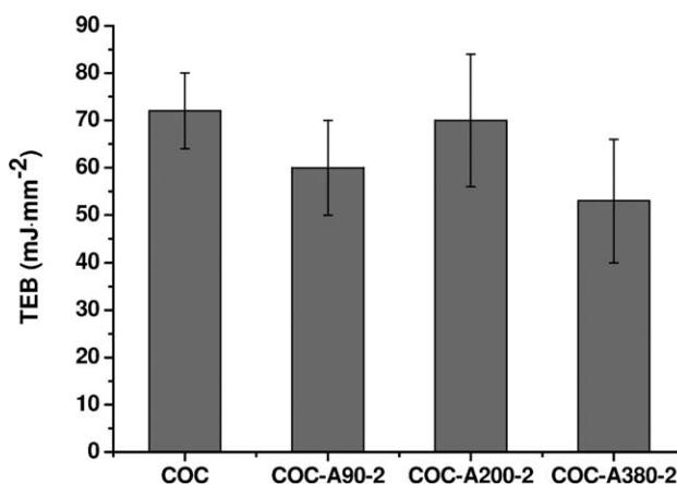
**Figure 7** Specific TEB of the neat COC and related nanocomposites under the tensile impact conditions ( $v = 1.25$  m/s).
