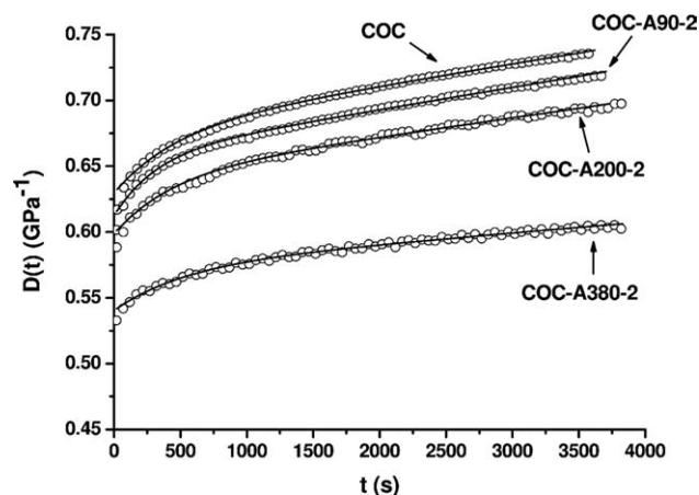
**Figure 9** Creep compliance data points for the neat COC and related nanocomposites (temperature = 30°C,  $\sigma_0 = 45\%$   $\sigma_{\max}$ ). The full lines fit the experimental data by the Burgers model.
