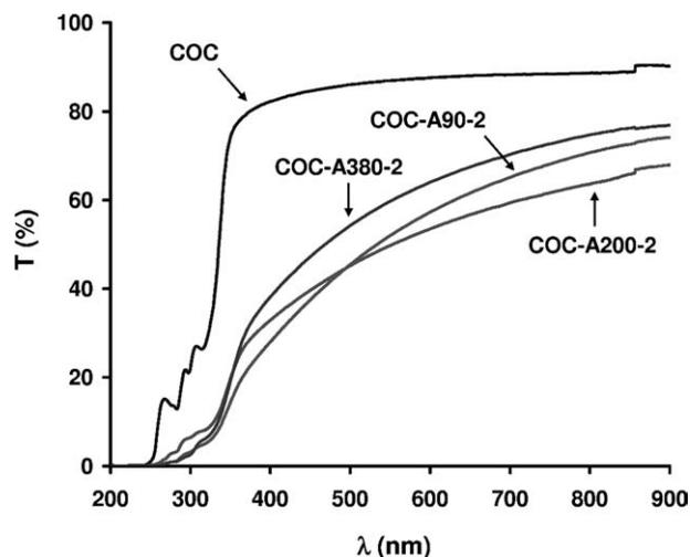
**Figure 10**  $T\%$  as a function of the wavelength of the neat COC and related nanocomposites.
