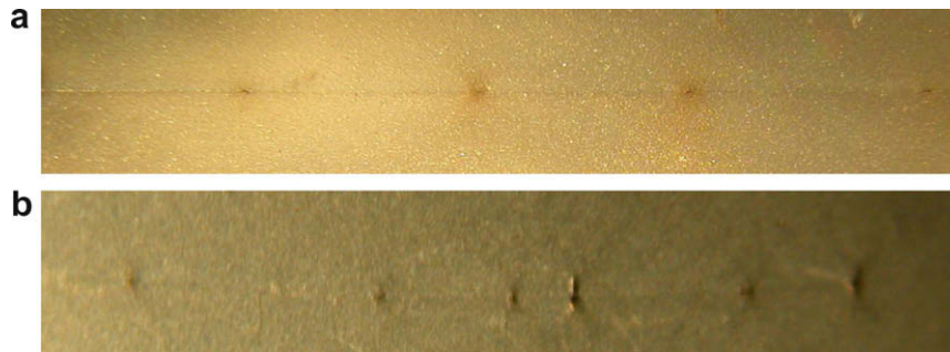
Fig. 6. Optical microphotographs (4 \times ) from fragmented fiber in microcomposites (a) M0.0 and (b) M1.0.
