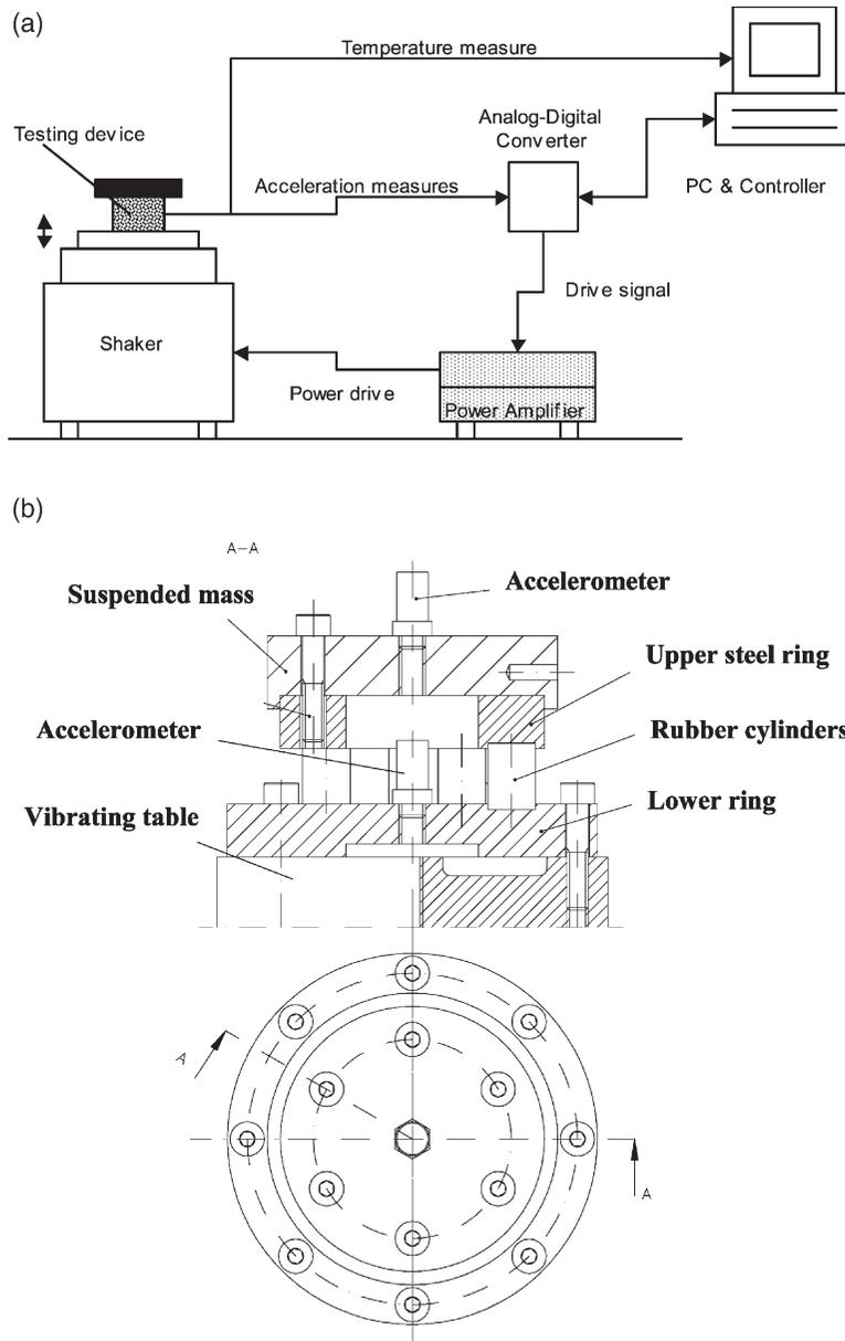
Fig. 1. Scheme of the apparatus (a) and test system (b) used for dynamic testing by ES.
