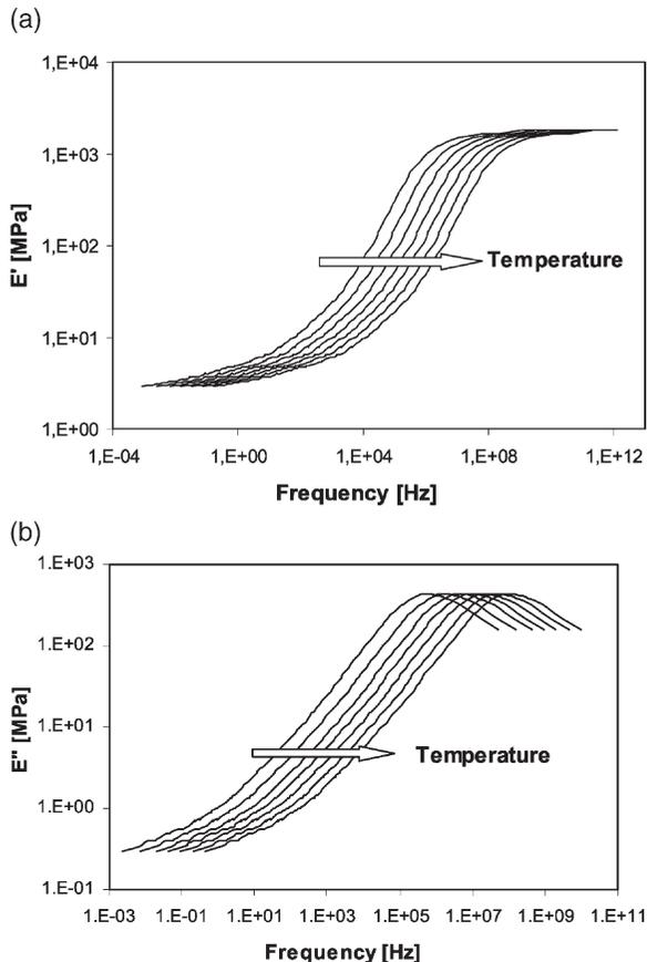
Fig. 4. Storage (a) and loss (b) modulus master curves of sample B for a strain amplitude of 0.7% at various reference temperatures (20, 25, 30, 35, 40, 45, 50°C).
