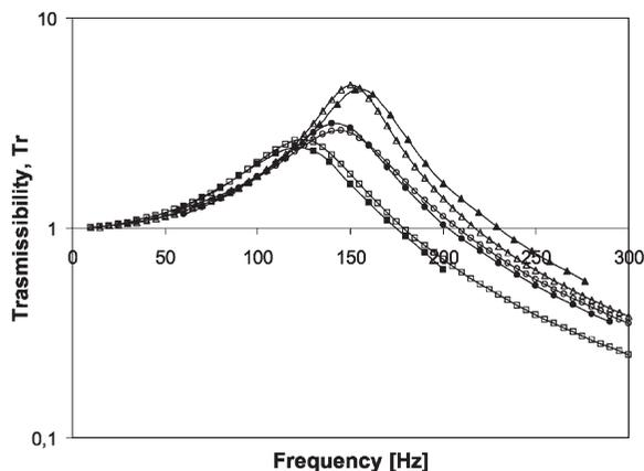
Fig. 10. Transmissibility of the test system, containing rubber test pieces of sample A, as a function of frequency. Data determined by ES testing (full symbols) and by dynamic moduli obtained by DMTA (open symbols) at different strain amplitudes ( $\blacktriangle$ , 0.2;  $\bullet$ , 0.5;  $\blacksquare$ , 0.7%).
