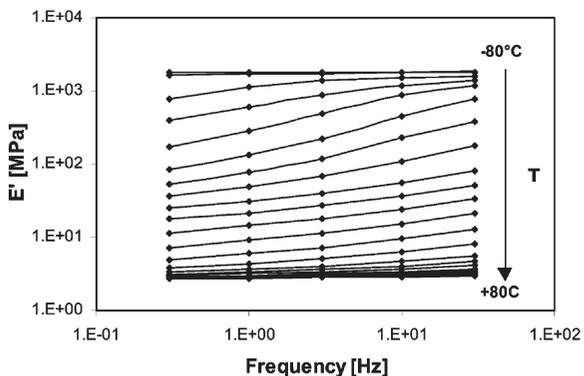
Fig. 3. Isothermal storage modulus values for sample B as a function of frequency, for a strain amplitude of 0.7%.
