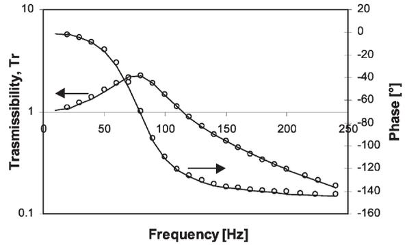
Fig. 6. Transmissibility and phase of the test system, adopted for ES testing, as a function of frequency. Rubber test-pieces of sample B. Data obtained by ES (full lines) and evaluated from dynamic moduli master curves obtained by DMTA (open circles).
