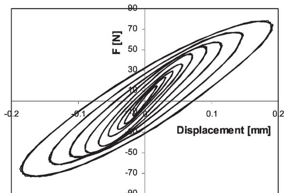
Fig. 9. Hysteresis loops for sample A determined by ES at various amplitudes of displacement.
