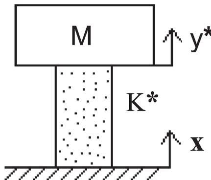
Fig. 5. Single degree of freedom system model.
