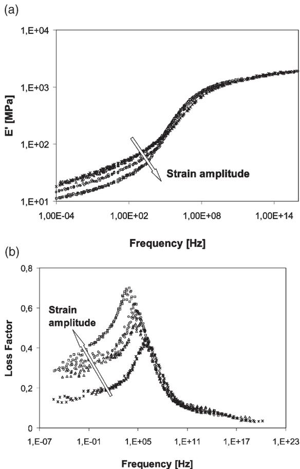
Fig. 8. Storage modulus (a) and loss factor (b) master curves of sample A for various strain amplitudes (×, 0.2; △, 0.5; ○, 0.7; □, 1.4%) referred to a reference temperature of 22°C.
