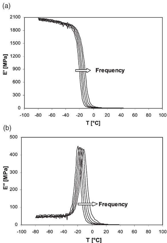
Fig. 2. Storage (a) and loss (b) modulus of sample B as a function of temperature measured by DMTA for a strain amplitude of 0.7% at various frequencies (0.3, 1, 3, 10, 30 Hz).
