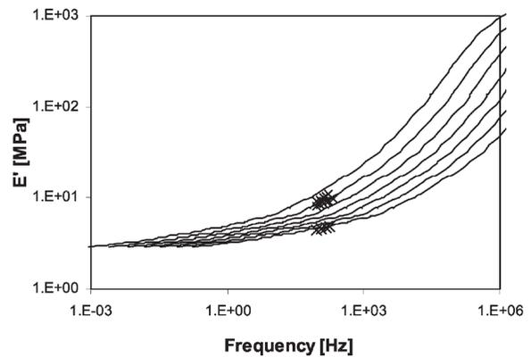
Fig. 7. Portion of storage modulus master curves of sample B at various reference temperatures (as shown in Fig. 4a). The values of  $E'$ , determined from transmissibility data obtained by ES testing at  $T = 25^\circ\text{C}$  and  $T = 50^\circ\text{C}$  are also reported ( $\times$  symbol).
