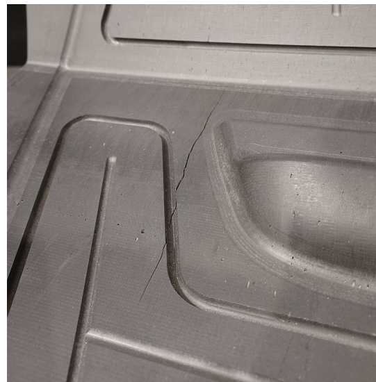
Fig. 2 Carbon fiber reinforced polyamide 6 trimming tool showing an interlayer crack growth developed during machining
