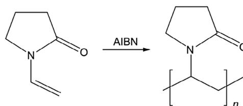
FIGURE 16 Synthesis of poly(vinyl pyrrolidone).<sup>[15]</sup>
