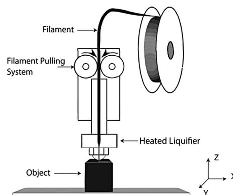
FIGURE 3 Fused deposition modeling technique (duplicated from Reference [28]).
