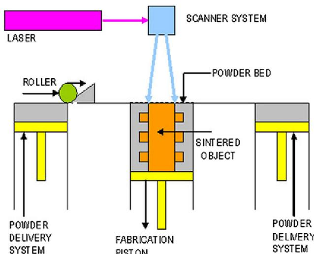
FIGURE 4 Scheme of selective laser sintering (duplicated from Reference [1,30]).
