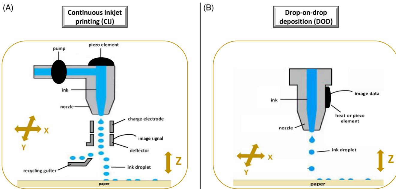
FIGURE 5 Scheme illustrating. (A) Continuous inkjet printing, and (B) drop-on-drop deposition techniques (duplicated from Reference [9]).
