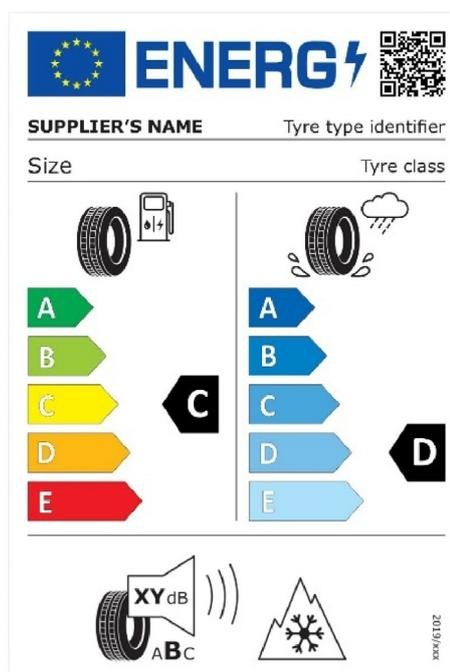
Fig. 2. New EU tyre labelling in accordance with Regulation (EU) 2020/740 [35].
