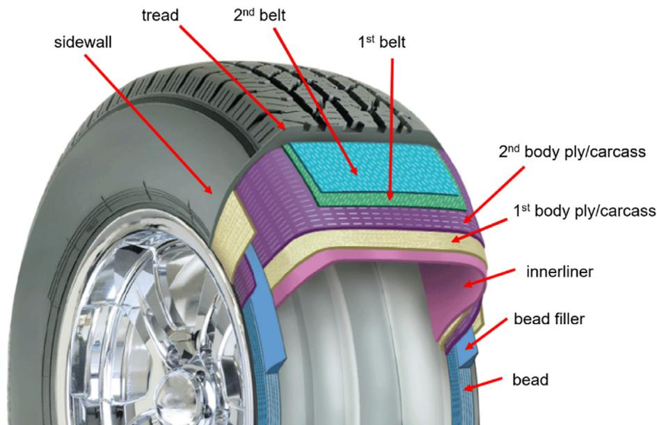
**Fig. 1.** Exploded view of a commercial passenger car tyre. Adapted from [15].
