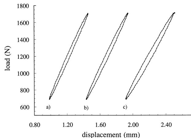
Fig. 8. Load–displacement hysteresis cycles for composite SENT specimens reinforced with 10 wt% of short glass fibres, tested at 0.1 Hz after (a) 240 cycles, (b) 690 cycles, and (c) 870 cycles.
