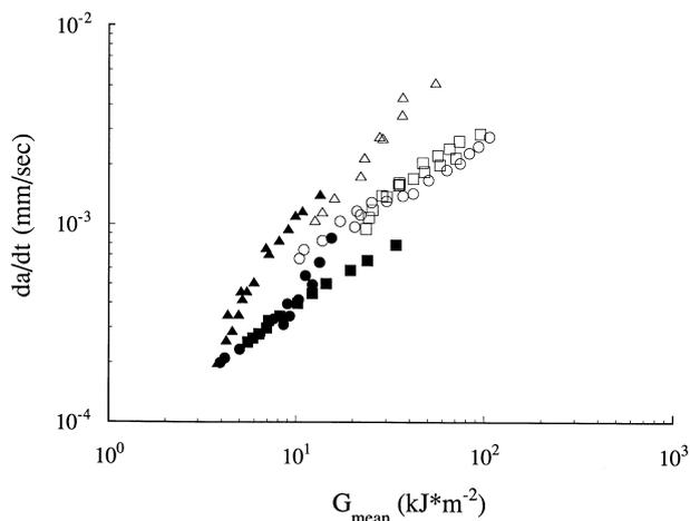
Fig. 7. Crack propagation speed,  $da/dt$ , as a function of the average strain energy release rate,  $G_{\text{mean}}$ , for composites reinforced with 10 wt% of short glass fibres, tested at ( $\square$ ) 0.1 Hz, ( $\circ$ ) 1 Hz, and ( $\triangle$ ) 10 Hz, and for composites reinforced with 30 wt% of short glass fibres, tested at ( $\blacksquare$ ) 0.1 Hz, ( $\bullet$ ) 1 Hz, and ( $\blacktriangle$ ) 10 Hz.
