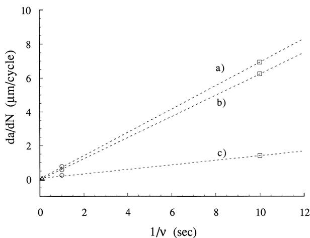
Fig. 6. Fatigue crack propagation rate evaluated at a constant  $\Delta K$  value of  $3.5 \text{ MPa}\sqrt{\text{m}}$  vs. the fatigue time period ( $1/v$ ) at ( $\square$ ) 0.1 Hz, ( $\circ$ ) 1 Hz, and ( $\triangle$ ) 10 Hz for composites reinforced with (a) 10 wt%, (b) 20 wt%, and (c) 30 wt% of short glass fibres.
