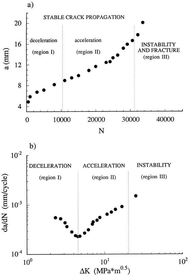
Fig. 3. Characteristic (a) crack extension,  $a$ , vs. number of fatigue cycles,  $N$ , and (b) crack propagation rate per cycle,  $da/dN$ , vs. stress intensity factor amplitude,  $\Delta K$ , curves for the short glass fibre reinforced polypropylene composites.
