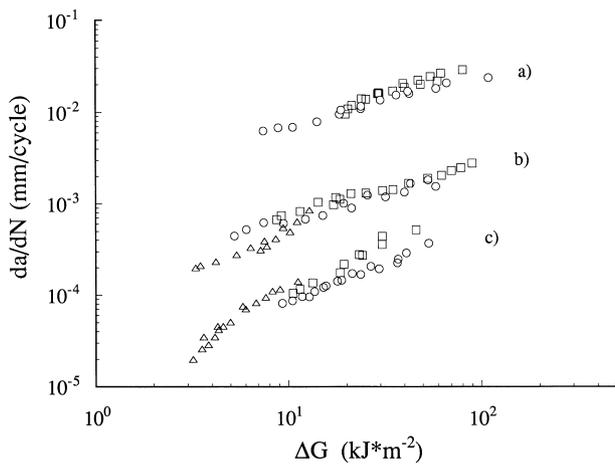
Fig. 5. Fatigue crack propagation rate vs. strain energy release rate curves at (a) 0.1 Hz, (b) 1 Hz, and (c) 10 Hz for composites reinforced with (□) 10 wt%, (○) 20 wt%, and (△) 30 wt% of short glass fibres.
