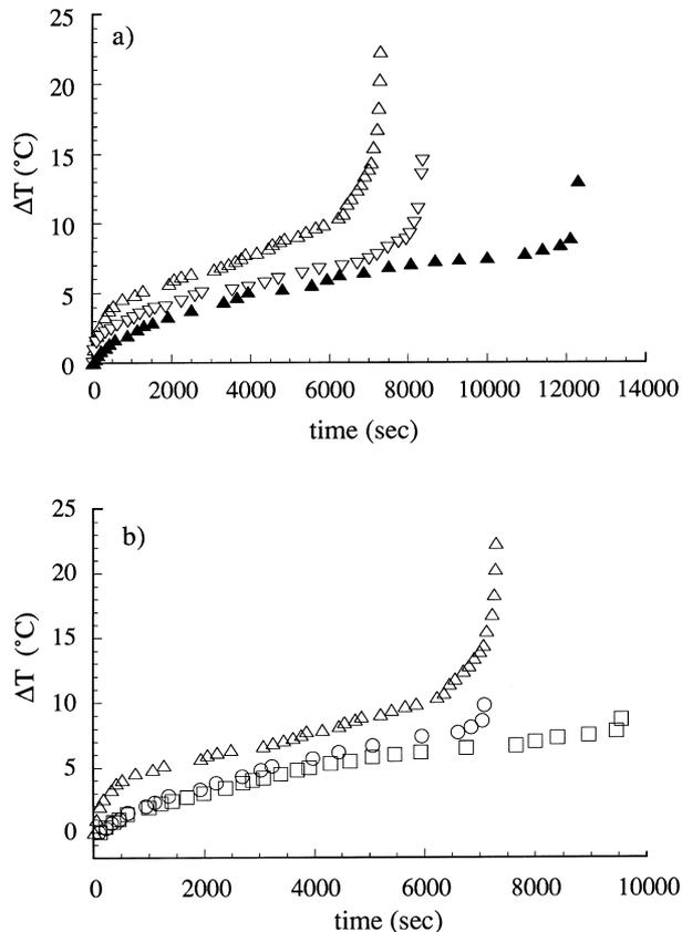
Fig. 10. Temperature increase at the crack tip during the FCP experiments for (a) specimens reinforced with (△) 10 wt%, (▽) 20 wt% and (▲) 30 wt% of short glass fibres tested at a frequency of 10 Hz and (b) specimens reinforced with 10 wt% of short glass fibres tested at (□) 0.1 Hz, (○) 1 Hz, and (△) 10 Hz.
