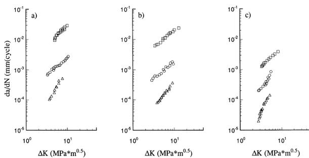
Fig. 4. Paris plots (stable crack acceleration region) at (□) 0.1 Hz, (○) 1 Hz, and (△) 10 Hz for composites reinforced with (a) 10 wt%, (b) 20 wt%, and (c) 30 wt% of short glass fibres.
