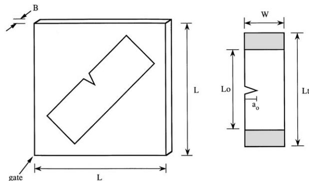
Fig. 1. Position from which test pieces were cut from polypropylene/glass injection moulded plaques, and shape and size of SENT specimens. Dimensions are:  $L = 127$  mm,  $B = 2.7$  mm,  $L_t = 120$  mm,  $L_o = 62$  mm,  $W = 27$  mm,  $a_0 = 3$  mm.
