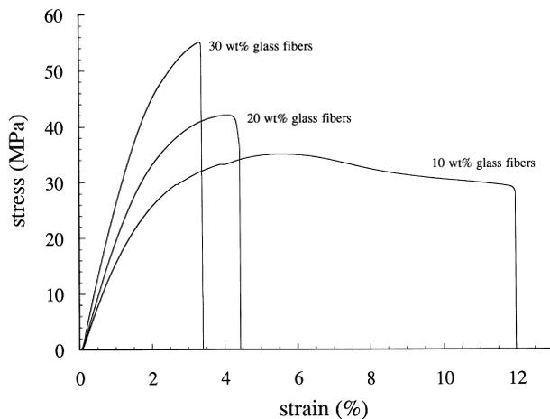
Fig. 2. Stress/strain curves of the short-glass-fibre-reinforced polypropylene composites used in the present study.
