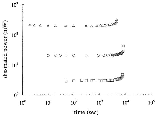
Fig. 9. Power dissipated in composite SENT specimen reinforced with 10 wt% of short glass fibres during the fatigue crack propagation at (□) 0.1 Hz, (○) 1 Hz, and (△) 10 Hz.
