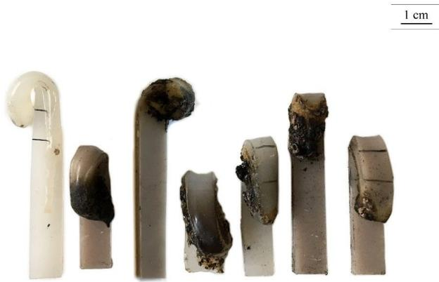
**Figure 10:** Samples after the LOI analysis. From left to right: PE, PE-HF-20, PE-HF-25, PE-Ar974-2, PE-Ar974-4, PE-HF-20-Ar974-2 and PE-HF-20-Ar974-5
