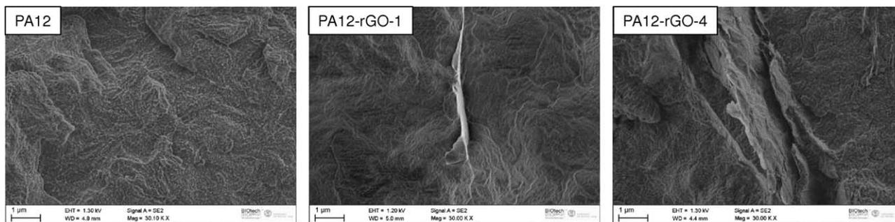
FIG. 2. FESEM images of the fracture surface of neat PA12 and of the relative nanocomposites (bulk materials).
