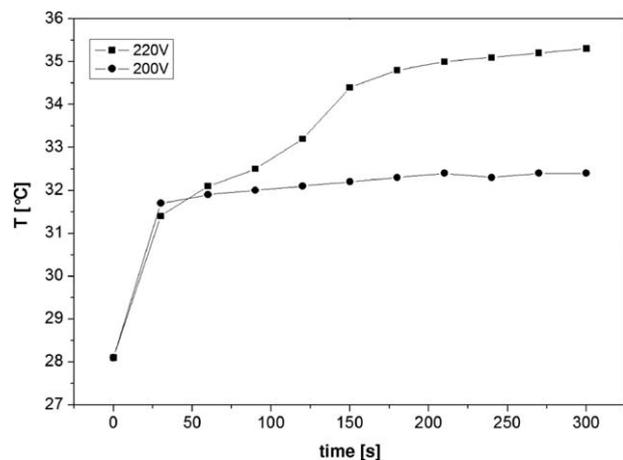
FIG. 9. Surface temperature evolution of the PA12-rGO-8 fiber with DR = 3 with an applied voltage of 200 V and 220 V.
