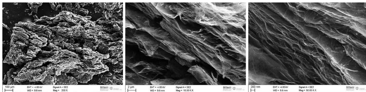
FIG. 1. FESEM images of the rGO powder at different magnifications.
