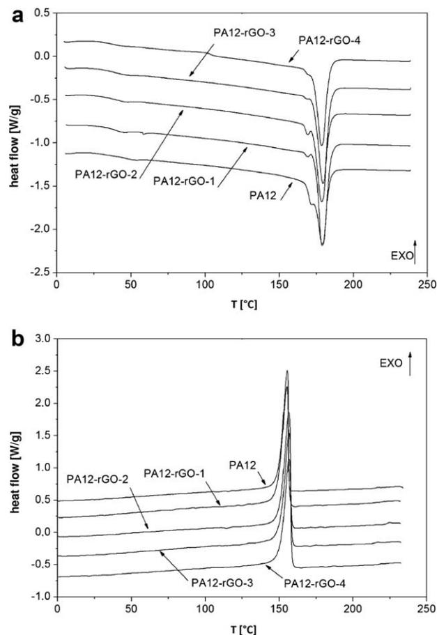
FIG. 3. DSC thermograms of neat PA12 and of the relative nanocomposites (bulk materials). (a) First heating stage, (b) cooling stage.
