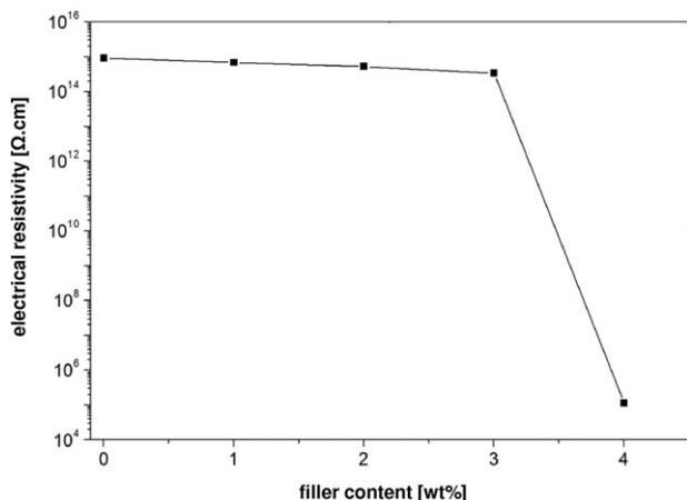
FIG. 6. Electrical resistivity values of neat PA12 and of the relative nanocomposites (bulk materials).
