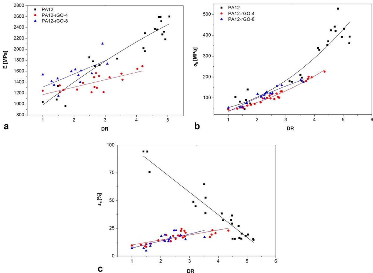
FIG. 8. Quasistatic tensile properties of PA12 and relative nanocomposites fibers as a function of the draw ratio. (a) Elastic modulus, (b) stress at break, (c) strain at break. [Color figure can be viewed at wileyonlinelibrary.com]
