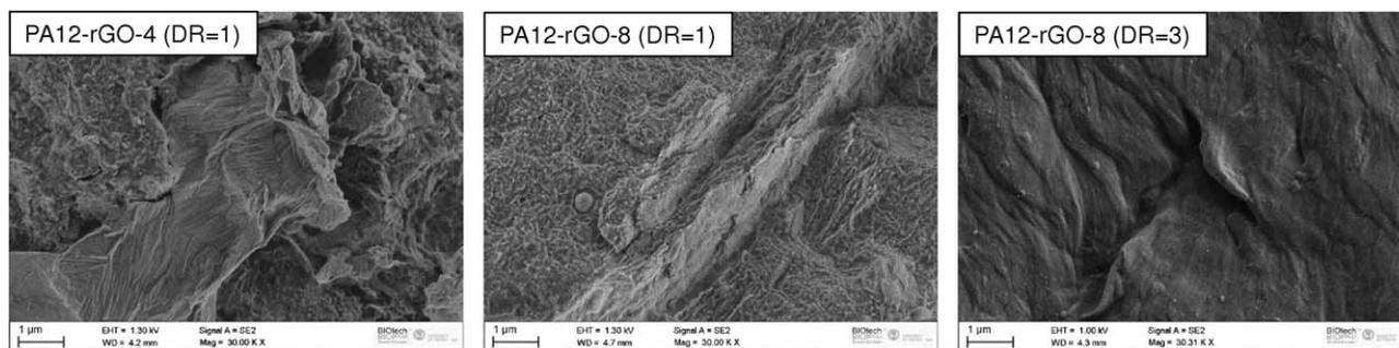
FIG. 7. FESEM images of the cryofractured cross section of PA12 based nanocomposites fibers.
