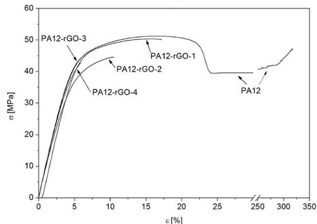
FIG. 5. Representative stress-strain curves of neat PA12 and of the relative nanocomposites (bulk materials).
