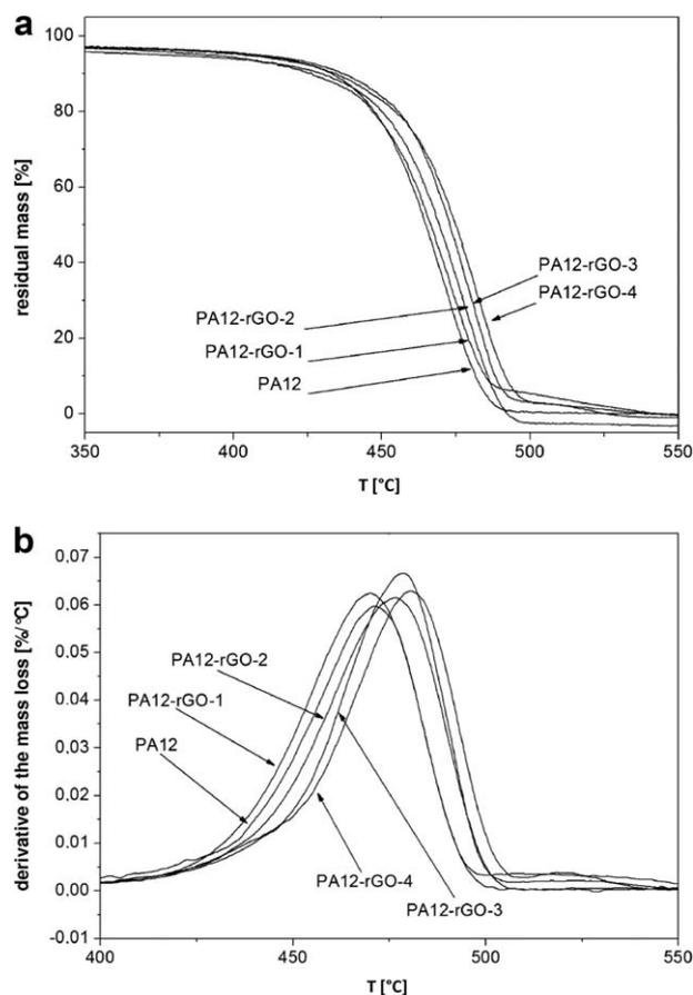
FIG. 4. Thermogravimetric curves of neat PA12 and of the relative nanocomposites (bulk materials). (a) Residual mass, (b) derivative of the mass loss.
