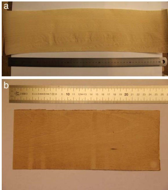
FIG. 1. Representative image of (a) a ultrathin wood lamina (thickness = 159 \mu\text{m} ) and (b) Comp-L laminate after hot pressing. [Color figure can be viewed at wileyonlinelibrary.com .]
