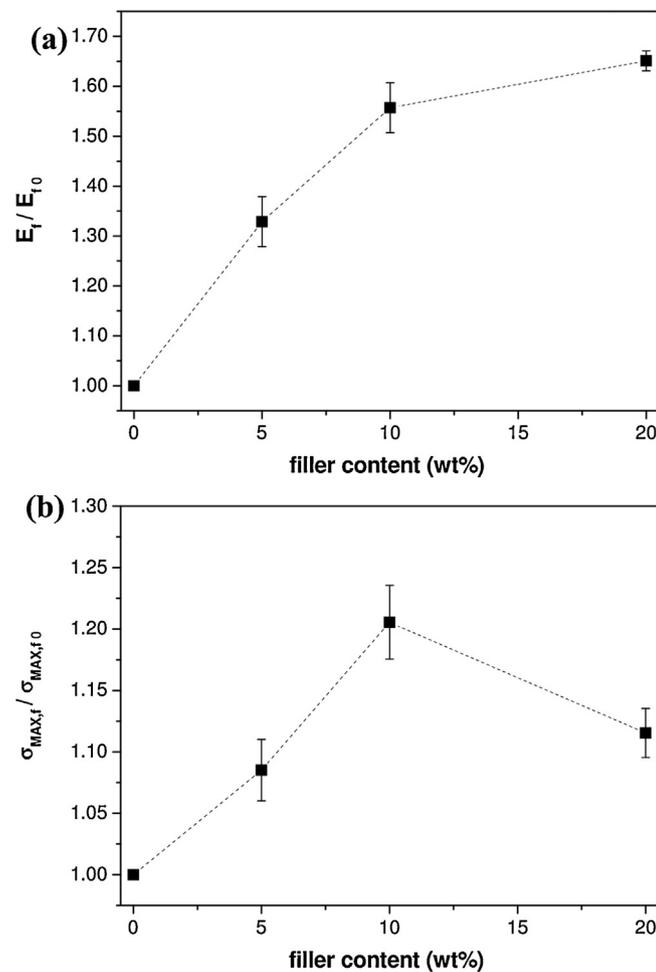
**Fig. 8.** Main relative flexure properties trends of neat photomatrix and corresponding microcomposites. (a) flexural modulus,  $E_f$ , (b) maximum flexural stress,  $\sigma_{MAX,f}$ .
