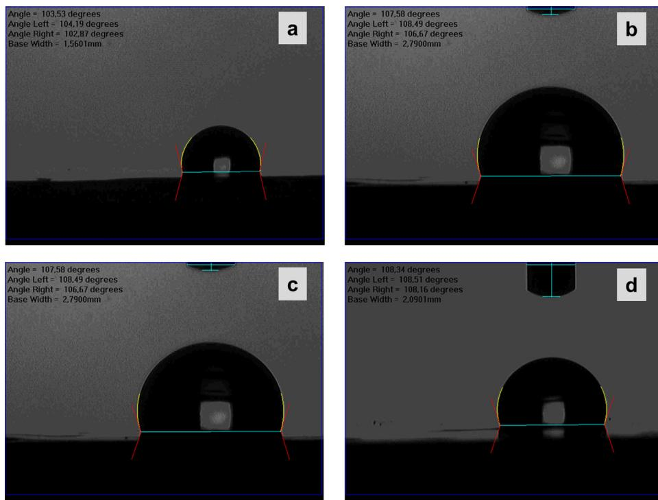
**Fig. 9.** Static contact angle of water on neat photomatrix and corresponding microcomposites.
