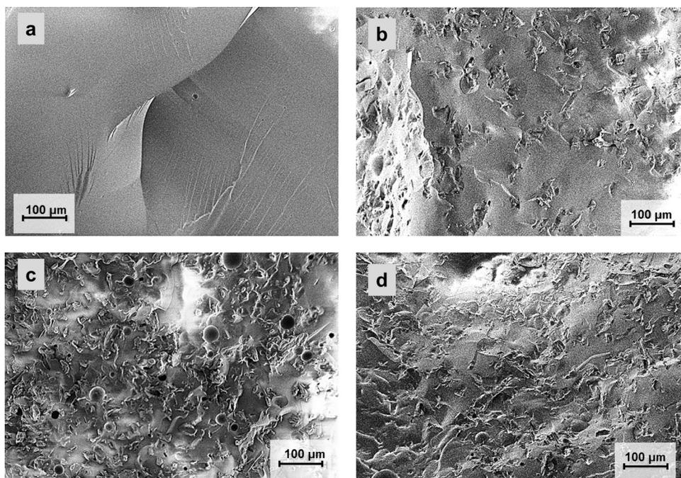
**Fig. 2.** FESEM images of the cryofractured surfaces of neat photoresin and corresponding microcomposites. (a) Photomatrix, (b) photomatrix-MCC-5, (c) photomatrix-MCC-10, (d) photomatrix-MCC-20.
