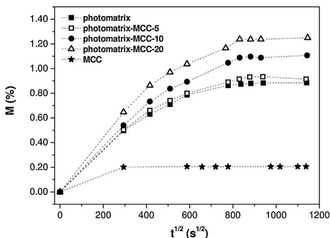
Fig. 10. Water uptake of MCC powder, neat photoresin and corresponding microcomposites conditioned at RH = 55% and T = 23 °C.
