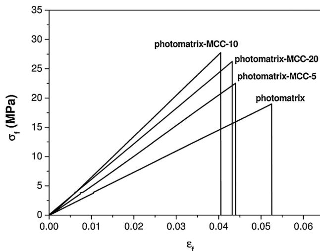
**Fig. 7.** Representative stress/strain curves of neat photomatrix and corresponding microcomposites from three points flexure tests.
