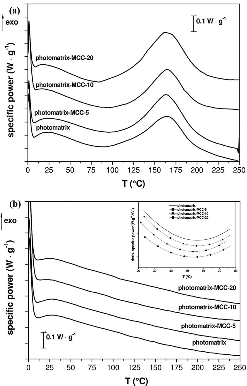
Fig. 4. DSC thermograms of neat photoresin and corresponding microcomposites. (a) First heating stage, (b) second heating stage.
