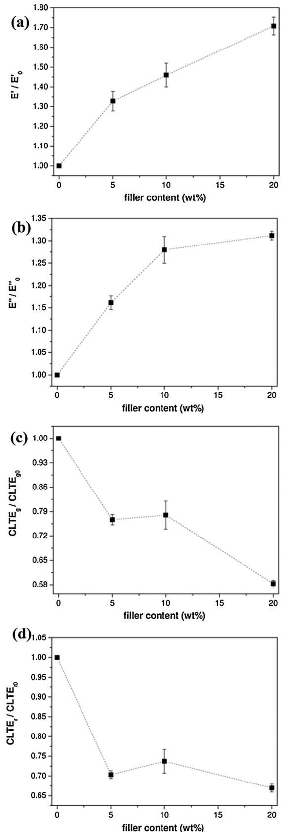
**Fig. 6.** Main results from DMTA analysis: (a) relative storage modulus,  $E'$ , (b) relative loss modulus,  $E''$ , (c) relative coefficient of linear thermal expansion below  $T_g$ ,  $CLTE_g$ , (d) relative coefficient of thermal expansion linear above  $T_g$ ,  $CLTE_r$ .
