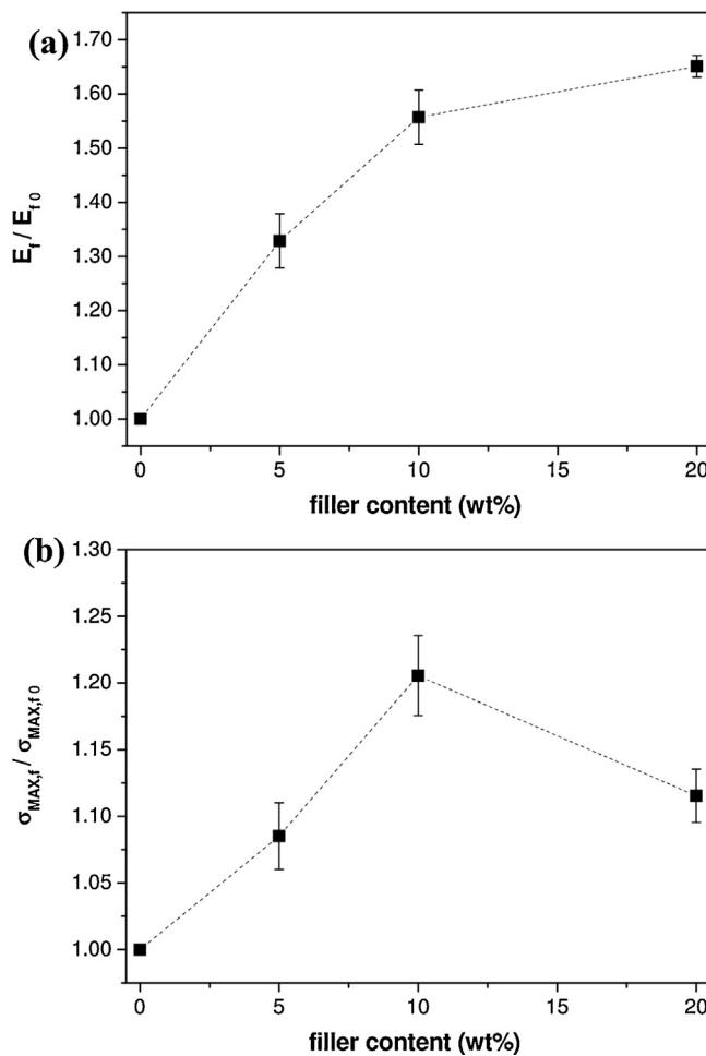
**Fig. 8.** Main relative flexure properties trends of neat photomatrix and corresponding microcomposites. (a) flexural modulus,  $E_r$ , (b) maximum flexural stress,  $\sigma_{\text{MAX},r}$ .
