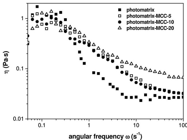
**Fig. 3.** Apparent viscosity of neat photomatrix and its corresponding microcomposites.
