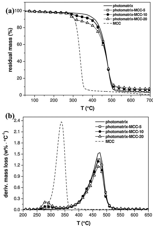
**Fig. 5.** TGA thermograms of neat photoresin, neat MCC, and corresponding microcomposites. (a) Residual mass as a function of temperature, (b) derivative of the mass loss.
