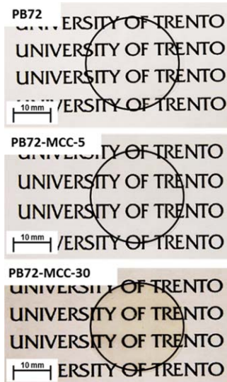
FIG. 2. Optical images of thin adhesive composite films showing the effect of the addition of 5 wt% and 30 wt% MCC on the optical properties of the PB72 matrix. [Color figure can be viewed in the online issue, which is available at wileyonlinelibrary.com.]
