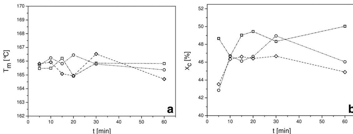
**Figure 4.** Results of DSC first heating scan on ( $\diamond$ ) PP-t, ( $\square$ ) PP-A200-t, and ( $\circ$ ) PP-R974-t samples ( $t = 5$ –60 min). (a) Melting temperature and (b) Crystallinity degree.
