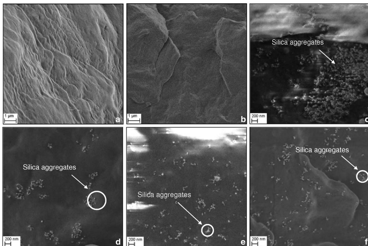
**Figure 2.** FESEM images of the fracture surfaces of (a) PP-5, (b) PP-60, (c) PP-A200-5, (d) PP-A200-60, (e) PP-R974-5, and (f) PP-R974-60 samples.
