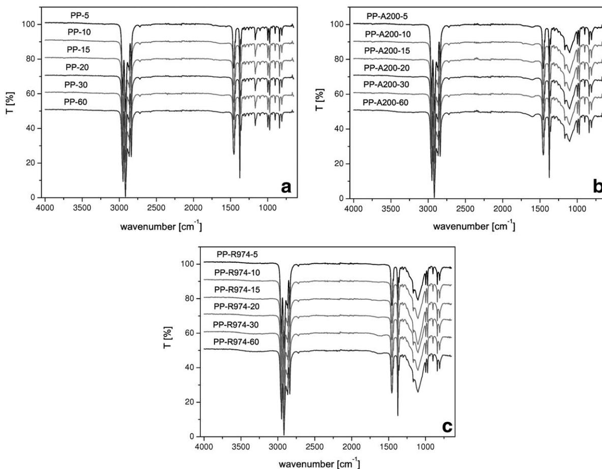
**Figure 3.** FTIR spectra of (a) PP-t, (b) PP-A200-t, and (c) PP-R974-t samples ( $t = 5$ –60 min).
