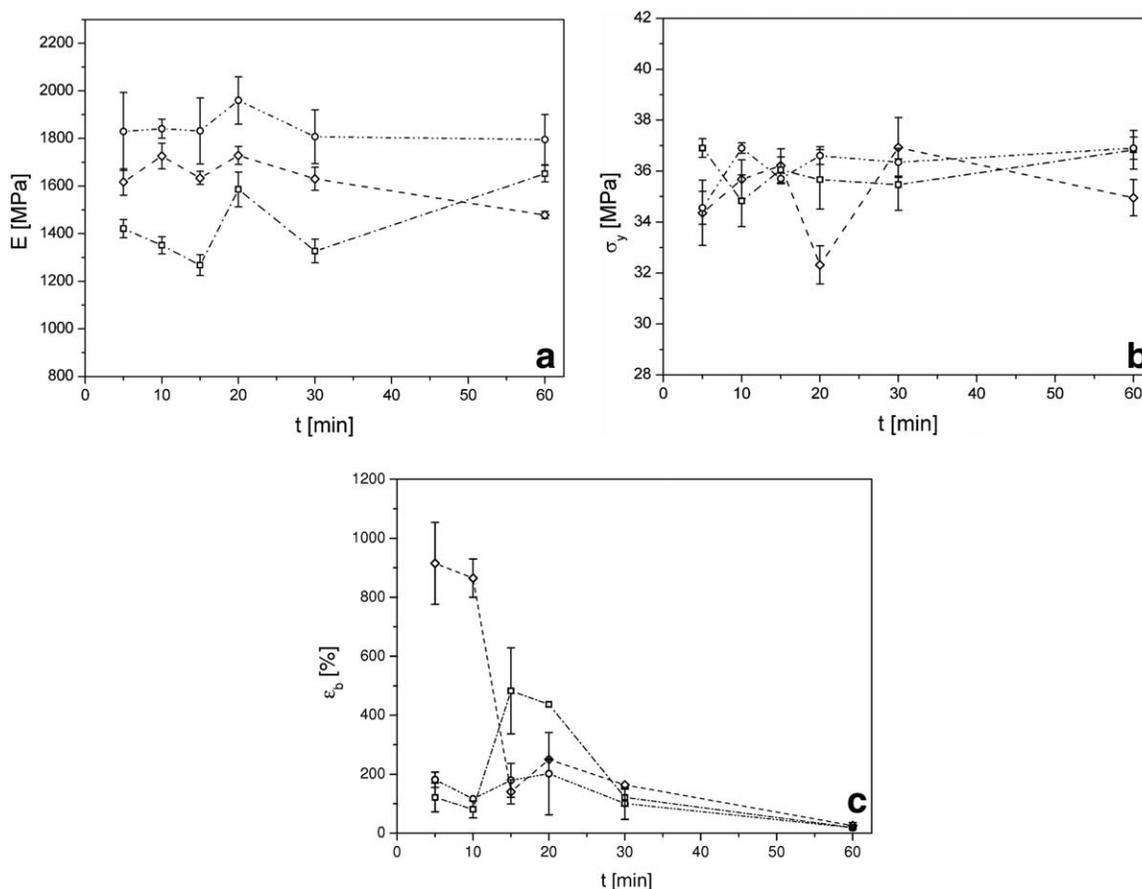
**Figure 6.** (a) Elastic modulus, (b) stress at yield, and (c) strain at break of ( $\diamond$ ) PP-t, ( $\square$ ) PP-A200-t, and ( $\circ$ ) PP-R974-t samples ( $t = 5$ –60 min).
