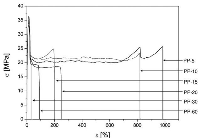
**Figure 5.** Representative stress–strain curves on PP-t samples ( $t = 5$ –60 min).
