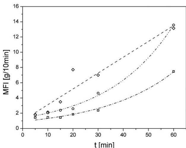
**Figure 1.** Melt flow index (MFI) values as a function of the processing time for neat PP-t (◇), PP-A200-t (□), and PP-R974-t (○) samples ( $t = 5$ –60 min).
