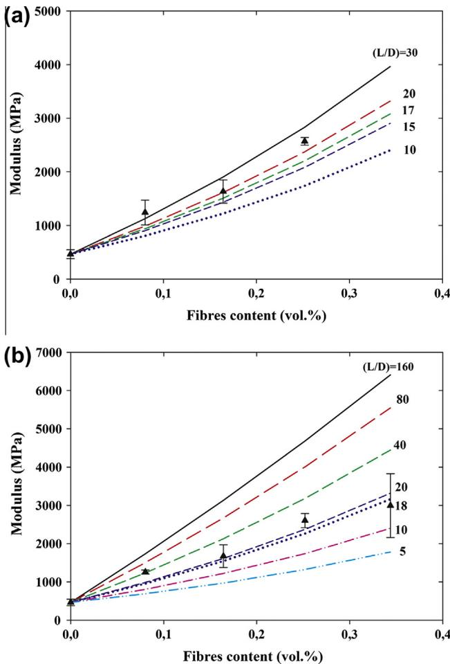
Fig. 6. Experimental ( $\blacktriangle$ ) and theoretical (lines) moduli values of G906PJ based composites reinforced by (a) SKF and (b) LKF. Predictions are based on the Halpin–Tsai model. (For interpretation of the references to colour in this figure legend, the reader is referred to the web version of this article.)
